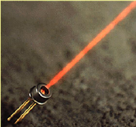
Vertical Cavity Surface Emitting Lasers are another device that relies on superlattices with nanometer thick films.
